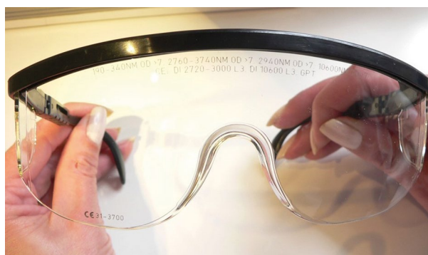
Fig. 12 Sample protective goggles, with reference to wavelength attenuation
