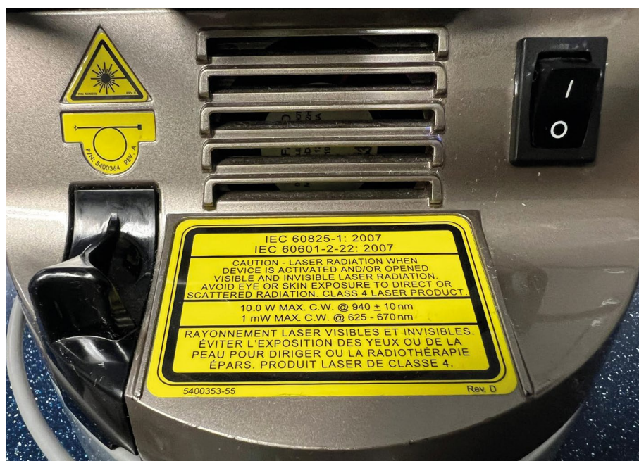
Fig. 7 Emission wavelengths – wavelength, emission mode and maximum power. Coaxial aiming beam is also referenced
