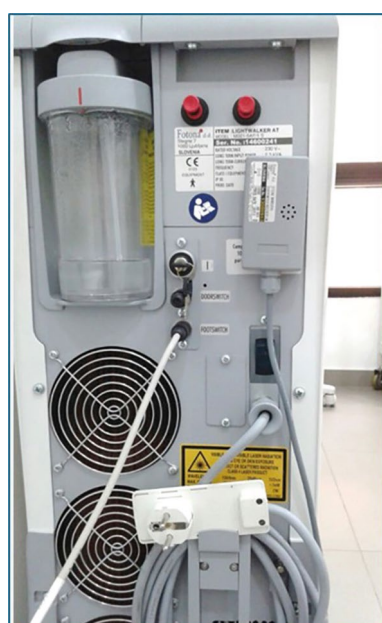
Fig. 9 Emergency STOP button to abort laser emission
