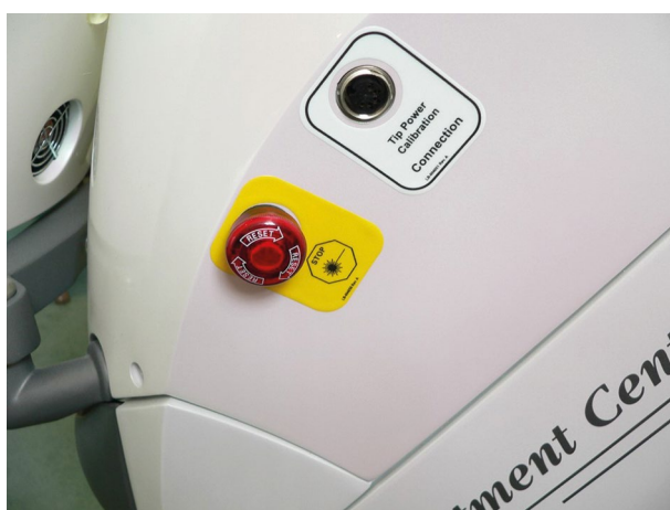
Fig. 9 Emergency STOP button to abort laser emission
